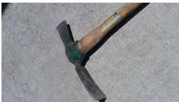
This tool has the axe blade at the top and the adze, the wide horizontal blade on the bottom.
